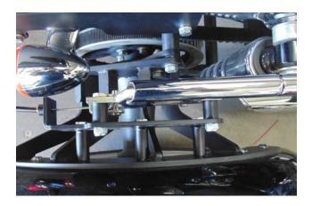
6. Mark the length of the housing. Cable needs to be longer than the housing. Do not cut the cable now. Remove housing from the cable. Use an abrasive cut off wheel to cut the housing. Do not Smash the housing
