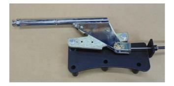
4. Slide cable housing over cable and locate front housing end in housing locator on the handle bracket.
