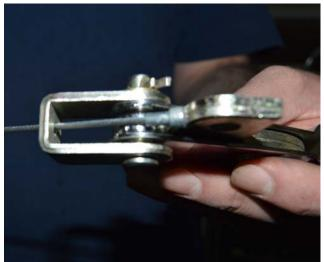
3. Bolt parking brake handle to handle bracket with supplied  $5/16'' - 18 \times 1 \frac{1}{2}''$  bolts and lock nut.
